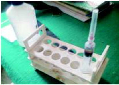
Fig 32 : Wrong practice of recapping the needle; Wrong practice of allowing blood to clot in the syringe itself. After collection, blood should immediately be transferred to the centrifuge tube and the tube should be allowed to stand for 20-30 minutes for clot formation, before centrifugation.
